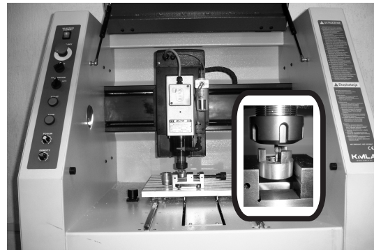
Fig. 1. Three axis milling machine used for testing the proposed algorithm.
